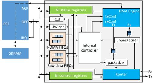
Figure 1: The AXIOM network interface architecture.
